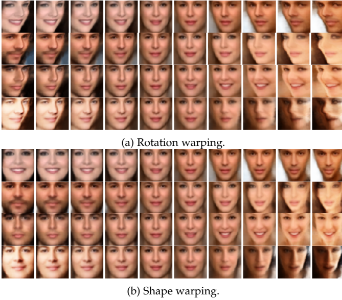
Fig. 5. Applying the geometric basis functions, (a) rotation warping and (b) shape warping, learned by the geometric generator to the canonical faces generated by the appearance generator. Compared with figure 3, only the pose information varies, and the identity information is kept in the process of warping.
