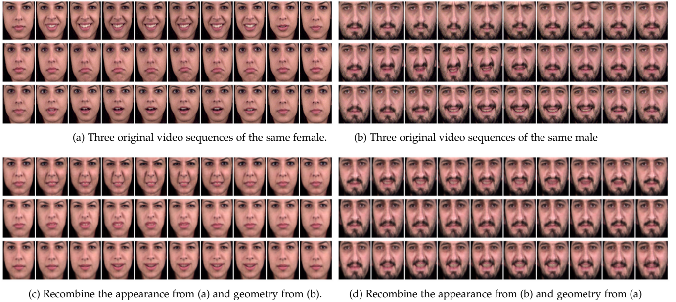
Fig. 13. Transfer and recombine the appearance and geometric information from different video sequences. (a) Three original video sequences of the same female with expressions of happiness, sadness and surprise; (b) Three original video sequences of the same male with expressions of anger, disgust, and happiness. (c) Transfer and recombine the appearance from female in (a), and the geometry from the male in (b), so that the generated video sequences in (c) inherit the appearance from the female but the shape and expressions (anger, disgust, and happiness) from the male. (d) Transfer and recombine the appearance from the male in (b), and the geometry from the female in (a), so that the generated video sequences in (d) inherit the appearance from the male but the shape and expressions (happiness, sadness and surprise) from the female.
